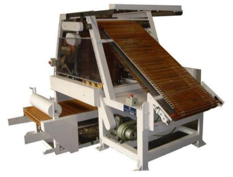
This is Cross Layer for putting Web on another from Sample Roller Card on Cross Layer Lattice. This Cross Layer Lattice is movable by  $90^{\circ}$  so that the Web can be made at will. The formed Web is put on one another to several levels on a purpose and a use.
