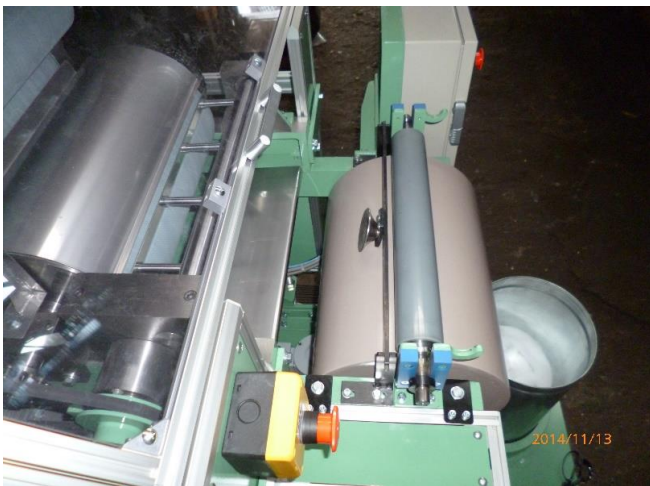
winding roller for web and simplified coiler for sliver
